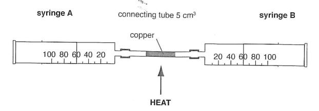
The teacher told the class that the volume of air in the connecting tube was 5 cm<sup>3</sup>. He also told them that the copper would react with the oxygen in the air.
