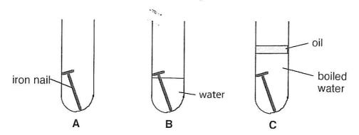
(a) (i) Suggest in which tube the iron nail would rust the most. (1)
