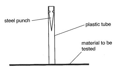
She decided to drop a sharp steel punch from the same height onto different materials and to measure the diameter of the mark in each material.
